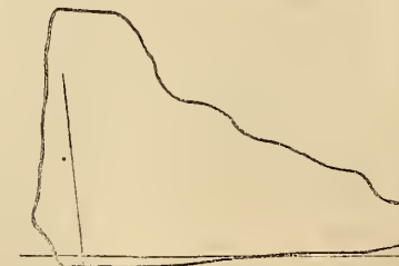
D. High-pressure—Bottom of Cylinder. Steam ..... 112 Vacuum ..... 18 Revolutions ..... 52
